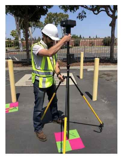
Control Target Coordinates are Determined by Survey Grade GPS or Traditional Survey Equipment
