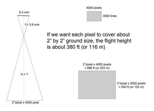
From the scale calculation formula, we know that UAS photos captured at 380 ft cover an area of 666 x 500 ft (or 203 x 152 m) Photo width: 4000 pixels x 2 inches/pixel = 666 ft (or 203 m)
